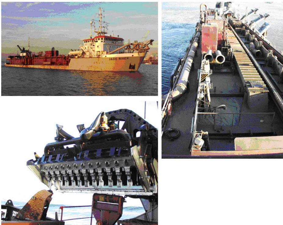
Figure 3. A few photographs of the trailing suction hopper dredger Jade River: trailing suction hopper dredger Jade River (above left), detail of the suction head (below left), and detail of the hopper (right) (Vos et al. 2009)
